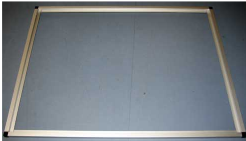
Step 2: The 4:3 frame for the glass screen surface is assembled.
