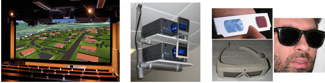
Figure 2: The Powerwall arena at the VR Media Lab (left). The projector system with polarized filters for the Powerwall system at the Aalborg University Copenhagen, Medialogy Lab (center). Goggles for 3D stereo visualization systems (right): red-cyan Anaglyph on white frame, Polarized filters on black frame, shutter glasses on gray frame.
